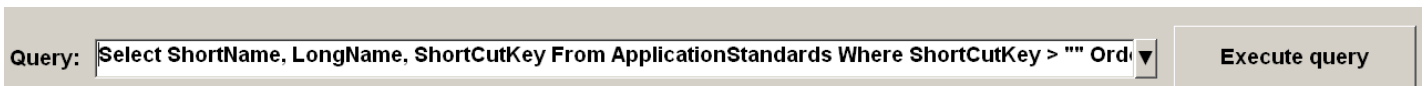
Figure 59: Enter the following command: Select ShortName, LongName, ShortCutKey From ApplicationStandards Where ShortCutKey > "" Order By ShortName
