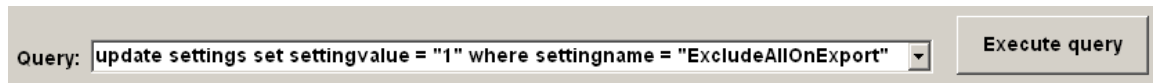
Figure 42: Enter the following command in the “Query” text box: update settings set settingvalue = "1" where settingname = "ExcludeAllOnExport"
