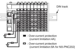
Applicable wire size for Unit power source and IO power source terminal
