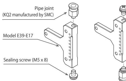
2. Attach to the sensor and insert the tube.
