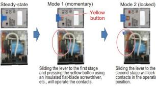
Sliding the lever to the second stage will lock the contacts in the operating position.
