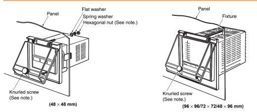
Note: Tighten the knurled screw to a torque of 0.02 N·m and the hexagonal nut to a torque of 0.05 N·m.
