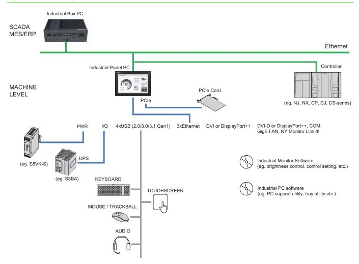
\*NY Monitor Link option: Connect monitor up to 100 m via Ethernet cable.
