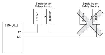
4. The total wiring length for the E3ZS Single-beam Safety Sensors is 30 m max.
