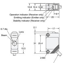
Vinyl-insulated round cord with four Receiver conductors and three Emitter conductors, 4 dia. (cross sections of conductors: 0.2 mm², insulation system: 1.1 mm dia.) Standard length: 2 m
