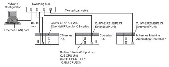
\* EtherNet/IP Unit with unit version 1.0 or later (Lot number 241001□ or later) is required to connect CJ1W-EIP21S to NJ-series CPU Unit. For lot numbers 241001□ or later, "+NJ" is printed at the lower right of the Unit's front panel.
