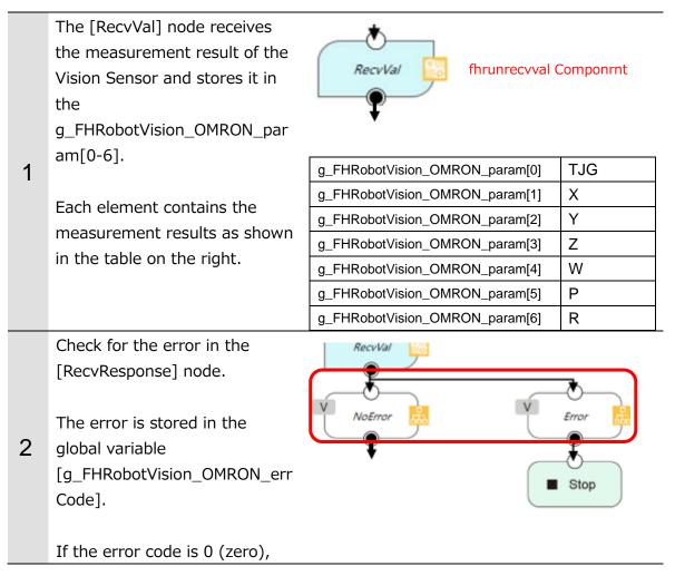
proceed to the next node. Check the TJG of the Vision V Sensor measurement result. If g\_FHRobotVision\_O 1 MRON param(0) The TJG of the Vision Sensor measurement result is stored in the global variable Stop 3 [g\_FHRobotVision\_OMRON\_pa ram[0]]. If TJG is OK (1), proceed to the next node, otherwise exit
