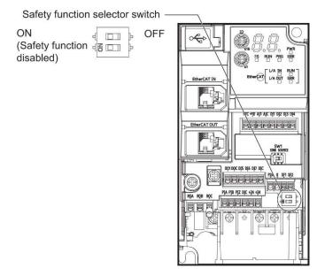
To activate Safety over EtherCAT (FSoE) on 3G3M1, change both switches on SW9 to ON (Left), like picture below.
