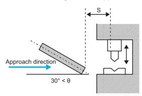
When the angle of the detection area exceeds ±30° with respect to the approach direction, the approach is considered as vertical approach and the calculation formula of A is applied.
