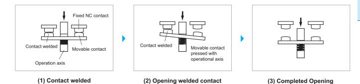
Contacts with direct opening action can be opened by applying the specified direct operating force (DOF) to the actuator to move it to the end of the direct operating travel (DOT) even when the force equivalent to the contact welding force (10 N) is applied in the direction of closing the contacts. The gap between open contacts must withstand the specified impulse voltage.
