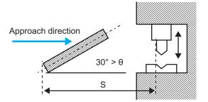
When the angle of the detection area is less than ±30° with respect to the approach direction, the approach is considered as parallel approach and the calculation formula of B is applied.
