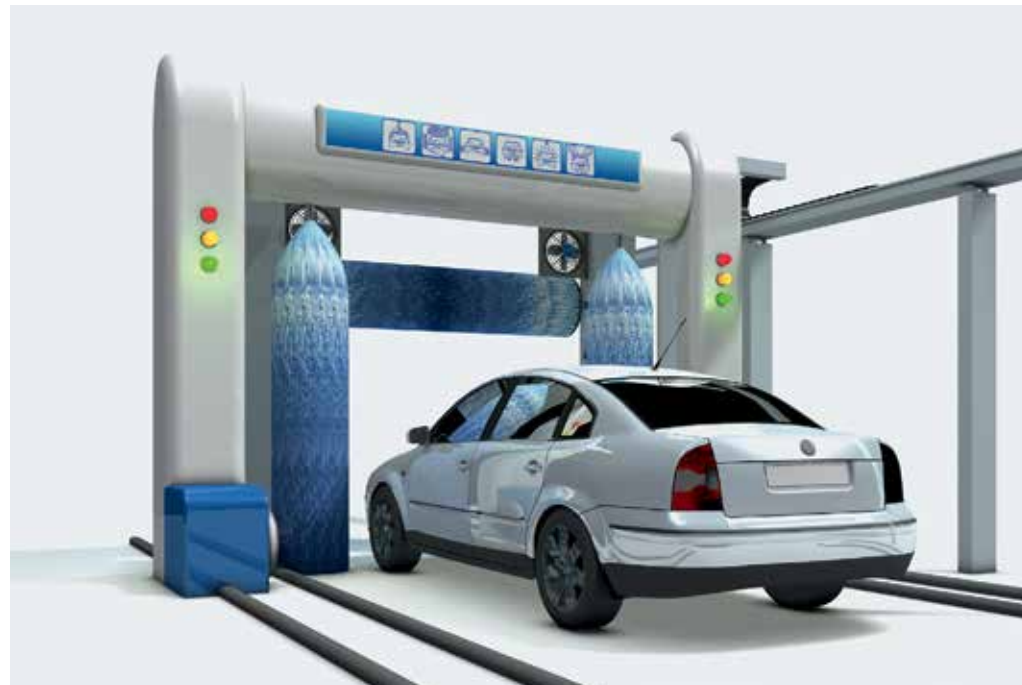
Car washing system. Proximity sensors control end positioning of the frame and also current position of wash brushes. The sensors should have a long life time to survive in high humidity and permanently changing external temperature.
