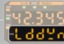
Equipped with a laser lifetime monitor to warn of laser deterioration.
