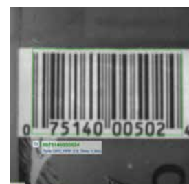
Polarizer – Eliminates glare
