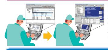
Previously, creating screens required typing in addresses for lamps and switches while looking at symbol tables (i.e., addresses, names, and comments). This resulted in typing mistakes in addition to having to input addresses for buttons and lamps twice. Importing the symbol tables solves the problem of wasted effort and typing mistakes to greatly reduce labor spent designing screens.
