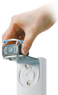
The reading angle of the code reader that is loosely screwed to the L bracket can be adjusted using the position adjustment holes.
