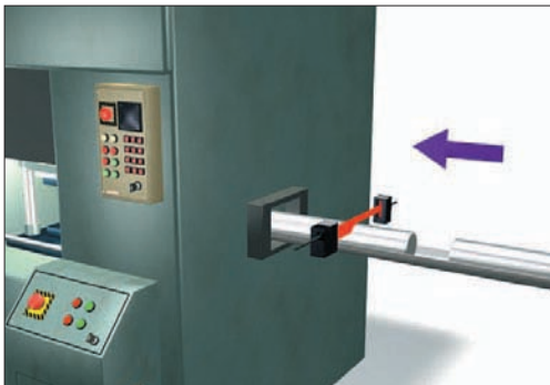
Diameter measurement of metal objects
