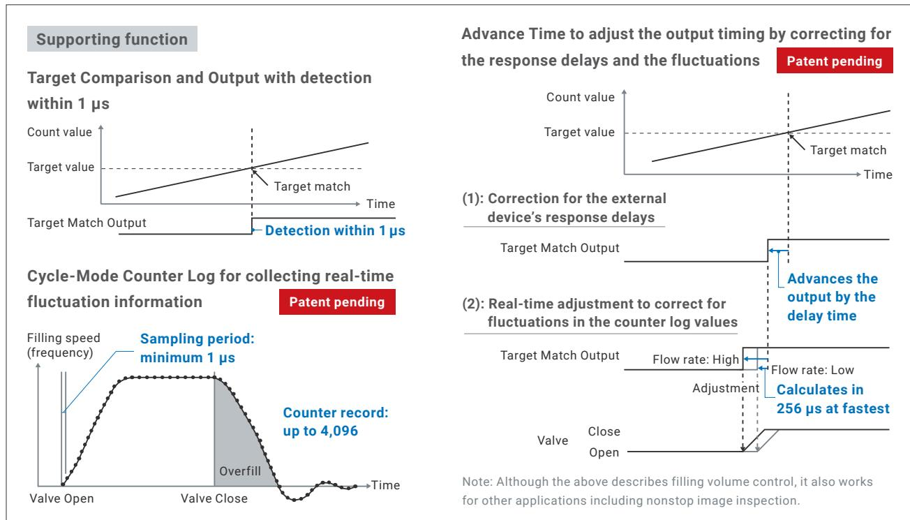
NX-CT features the Counter Comparison function with detection within 1  $\mu$ s. It achieves high-speed, high-precision control through lightning-fast edge control, which processes signals instantly within the unit. It can reduce waste and loss on production sites caused by control delays, and contribute to production environments that can maximize added value.
