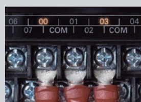
Input/output terminal LED indicators for quick troubleshooting
