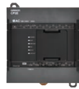
CP2E-N CPU unit with 14 or 20 I/O points
