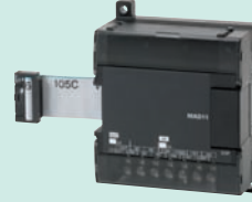
CP1W-MAD11 Analog inputs: 2 (resolution: 6,000) Analog outputs: 1 (resolution: 6,000)
