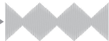
The image of the leakage current waveform at the secondary side of an inverter.
