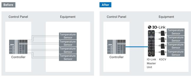
Reduces wiring between control panels and equipment
